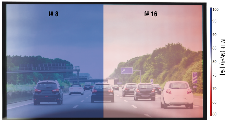
Left and right image of an ADAS camera system taken with different lens apertures. The corresponding MTF maps are overlaid.
