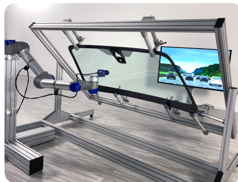
Automotive Imaging on a windscreen test bench and applied from inside of the car.
