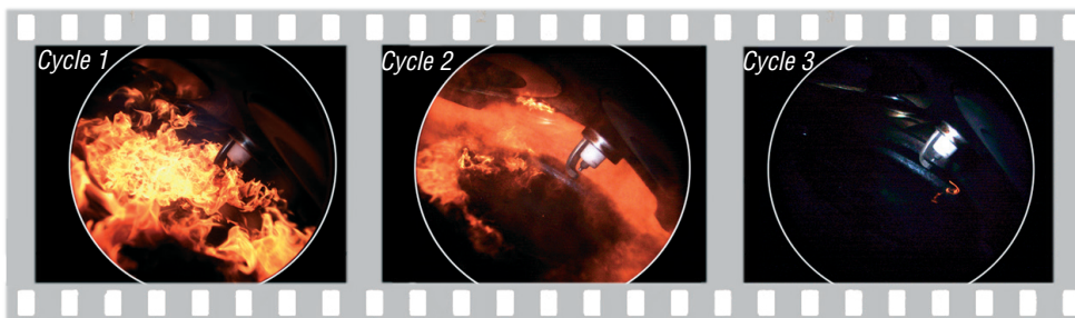
Soot formation in GDI engine during first cycles of a cold start at fixed crank angle position
