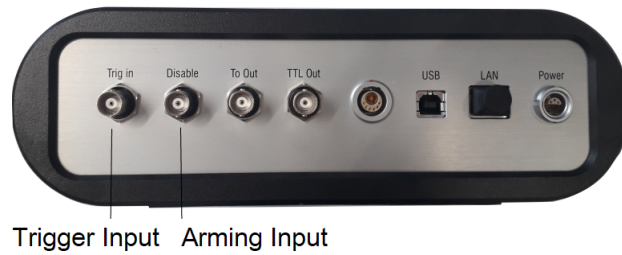
Figure 4.2: HS- IRO back panel: Connect the "Arming" signal to the "Disable" connector.
