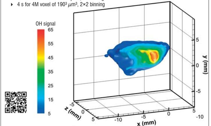
Figure 4: Iso-surfaces of OH-LIF intensity.  $Re_{jet} = 3200$ ,  $T_{co-flow} = 1050$  °C
