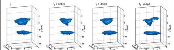
Figure 7: Time series of an auto-igniting CH<sub>4</sub> flame.  $Re_{jet} = 3200$ ,  $T_{co-flow} = 1050$  °C
