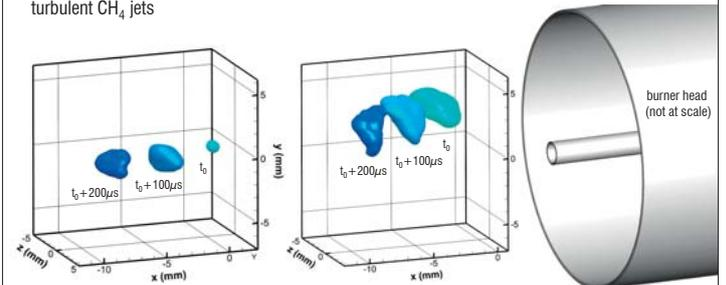
Figure 6: Propagation of auto-igniting kernels: overlay image of multiple time steps.  $Re_{jet} = 3700$ ,  $T_{co-flow} = 1100$  °C
