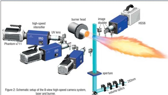
Figure 2: Schematic setup of the 8-view high-speed camera system, laser and burner.
