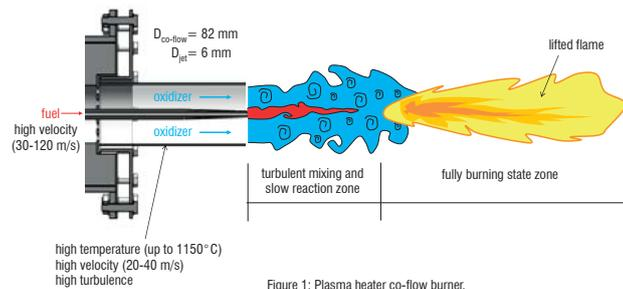
Figure 1: Plasma heater co-flow burner.
