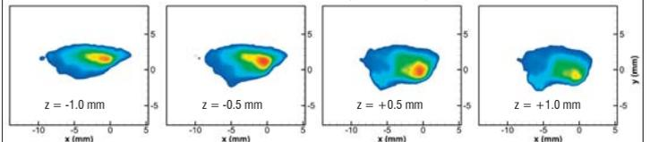
Figure 5: Reconstructed z-planes of OH-LIF from a flame kernel.  $Re_{jet} = 3200$ ,  $T_{co-flow} = 1050$  °C
