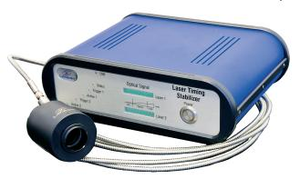
The **Laser Timing Stabilizer** consists of a fiber coupling mechanics which is mounted directly at the laser exit. A stable optical fiber leads the collected light to a controller where a fast photodiode measures the inherent time separation of the laser pulses.
