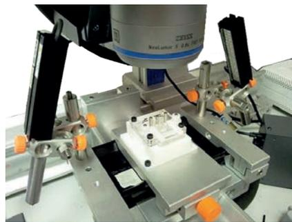
Where working distances are restricted or optical access is limited LaVision can provide small, divergent or collimated illumination units. Both units can also be run in a pulsed or constant illumination mode and their compact form factor allows them to illuminate sample surfaces even when optical access is restricted by either the microscope objective, or narrow windows in test chambers.
