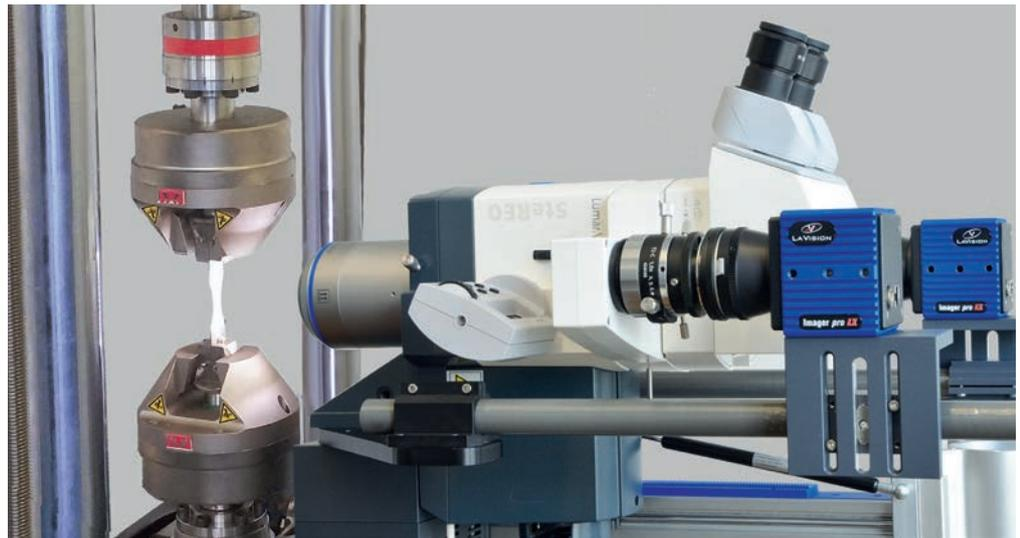
In addition to custom mounting arrangements systems can be configured with 1-3 axes of motorized translation, allowing motorized control of the area of interest and the focal plane. When working at the  $\mu$ -scale fine control of these parameters becomes very important and LaVision's tried and tested configurations can save users hours in setup time.
