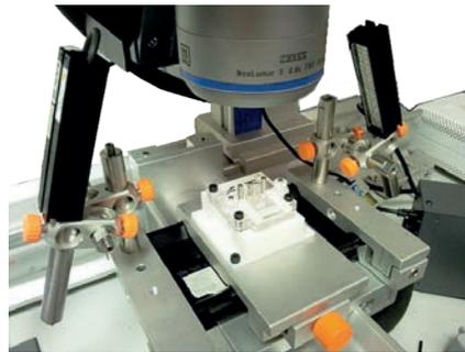
Where working distances are restricted or optical access is limited LaVision can provide small, divergent or collimated illumination units. Both units can also be run in a pulsed or constant illumination mode and their compact form factor allows them to illuminate sample surfaces even when optical access is restricted by either the microscope objective, or narrow windows in test chambers.
