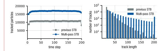
Two major improvements of the **Multi-pass** method can be seen, here. Firstly, the number of simultaneously tracked particles for the **Multi-pass** approach clearly surpasses the number for the previous implementation. Secondly, the particles can now be tracked three times longer, on average, with the new **Multi-pass Shake-the-Box**.
