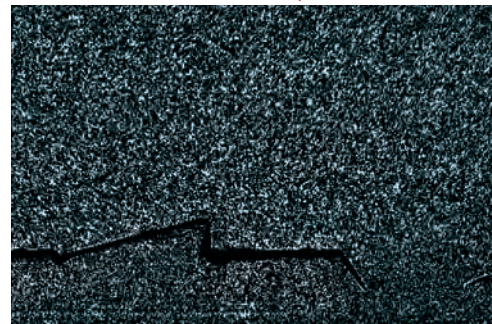
Processed image, courtesy: F. Scarano, A. Sciacchitano, TU-Delft, ARIANE V main engine, in: Robust elimination of light reflections in PIV, PIV'11, Japan
