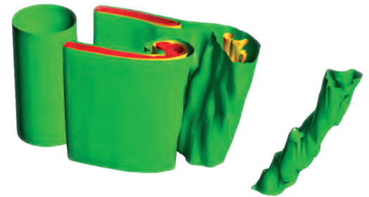
3D Reconstruction: the vorticity field is reconstructed in three-dimensions using a time-resolved phase averaging approach with POD and LDV phase reference signals.
