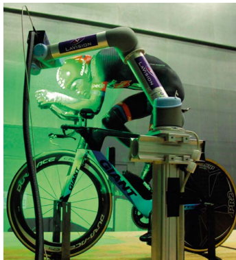
At TU Delft the flow field surrounding the complex shape of a human-sized mannequin and a racing bike was obtained with the MiniShaker TR-S mounted to a robotic arm and with co-axial laser illumination, courtesy TU Delft.
